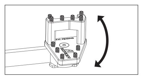
(4) Check brake pedal movement to be sure there is no interference with other parts of your bike. If the riser is installed, adjust your brake pedal height so that in the seated position you are using the enlarger, while in the standing position you will use the riser. Adjust your pedal height using the manufacturer's instructions to ensure correct procedure. It is important to set the correct free play to avoid caliper drag and potential brake failure.
