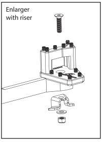
Place enlarger on brake pedal tip. Insert M5 x 35mm screw, and use 8mm socket tool to attach steel lower plate with M5 washer and M5 locknut. Tighten to 4.4Nm.
