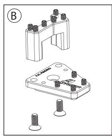
(A) If your kit is equipped with the optional Riser, install the grip pins with thread locker in the riser now.
