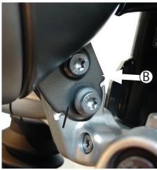
(A)Use 13mm socket and (B) T40 torx tool to loosen both mounting nuts and screws.
