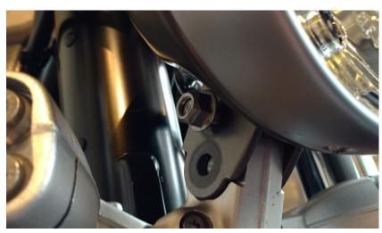
Remove the lower screw, and make sure the upper screw is only finger-tight.
