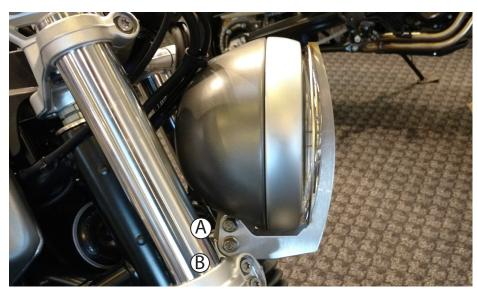
Support the headlight bucket by hand, or use painter's tape to secure in place.
