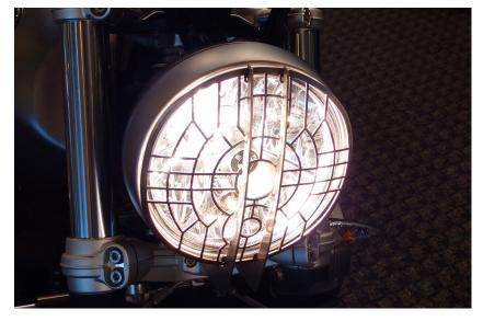
(5) Check headlamp aim based on your marks from step 1, and in accordance with manufacturer's instructions. Tighten both nuts to 20 Nm.
