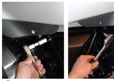
(1) Use 18mm socket and T55 torx to remove the engine through bolt. You will not reinstall this bolt.
