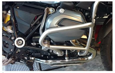
Adjust the bar location for good fit. Tighten the M6 screws to 7.5Nm. tighten the M12 nut to 85Nm
