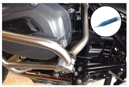
3 Attach the clamps to the left and right side. Add a drop of thread locker to the tip of each screw. Insert M6 x 35 screw with washer through both clamp halves and into the threaded hole in the tube flange.
