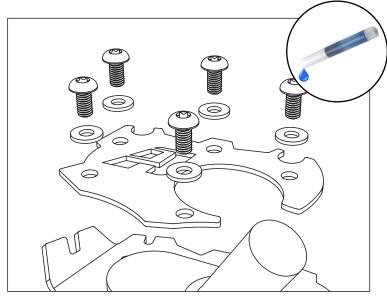
Take the (5) screws and add the washers and a small drop of thread locker to each screw. Now match up the bottom plate to the top plate and install all (5) screws with washers. Do this in the order shown in the picture.
