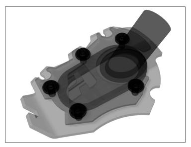
With bike on the center stand, arrange the top and bottom plates identically to how they are shown in the picture to get an idea of the fitment. Leave top plate resting on side stand.
