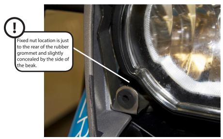
(6) Insert the cap head bolt with metal and then rubber washer from the bottom up. The bracket contains a fixed nut that you will thread into. Add a small drop of thread locker to the bolt before starting.
