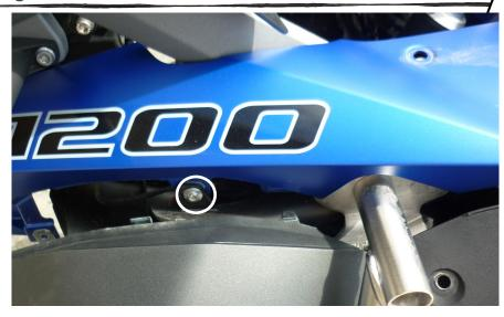
Gently peel back vent fairing to reveal (1) fastener on each side. Using T25 driver, remove the fastener from each side. Set aside for re-install later.
