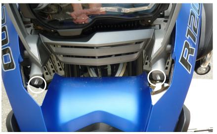
(6) You can now carefully remove the beak. Take note that there are two stand-offs in the front with rubber bushing that can come loose and fall out. You do not want to lose these.
