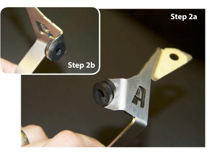
Install the (4) rubber grommets on the right and left side brackets. Sometimes it is easier to get grommets in place if you use some water as lubrication. You can also gently press into place with a flat head screwdriver.
