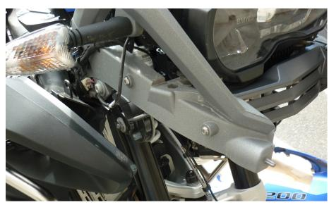
Resume normal headlight guard install by placing the spacers in the existing hole. Jump back to page 2, step 4. Re-install the beak and hardware after completing step 8.
