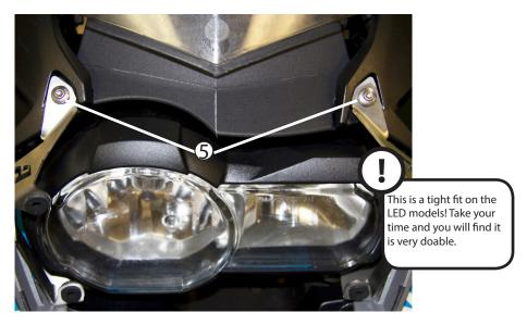
Install brackets with small clear round protective plastic between bracket and fairing on top mounting position. Install the (2) OEM T25 fasteners a couple of turns, do not tighten all the way.
