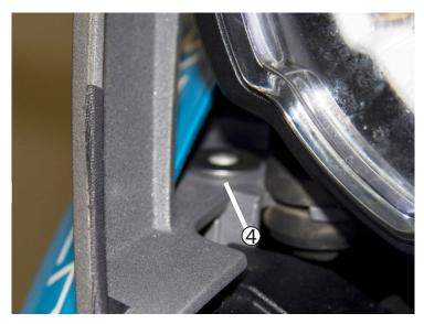
If you are working on a GS Adventure, skip to page 5 (if removal of beak is necessary to drop in spacers). Drop in (2) hat spacers, one on each side. The hexagonal hole the spacers go in is directly behind the beak fairing.
