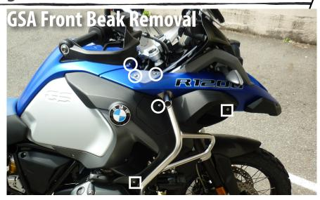
Using T25 driver, remove 6 fasteners from each side, 12 total. Be careful not to lose any spacers or protective plastic washers when removing fasteners. See all hardware aside for re-install later. Squares indicate long shoulder fasteners.
