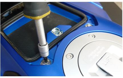
② Open up small storage compartment on top of gas tank and using T25 driver remove the (2) fasteners. Will be re-installed later.
