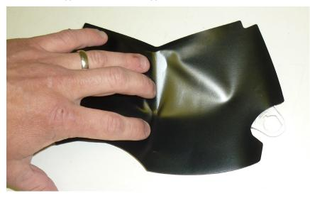
Attach sticker starting with the center ridge. The sticker is larger than the deflector and there should be some overhang on the edges. Press into the crosswise bend. Use your finger to press into place, pulling on the sticker edge with your other hand as necessary.
