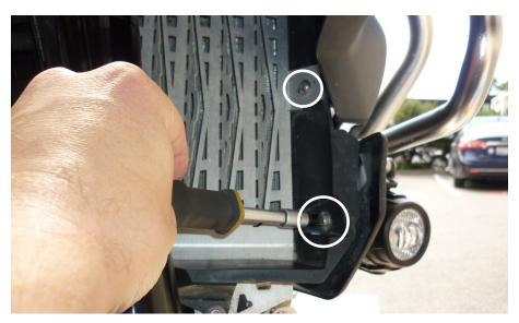
Using T25 driver, remove the (2) fasteners on each side, (4) total. Set aside for re-install later.
