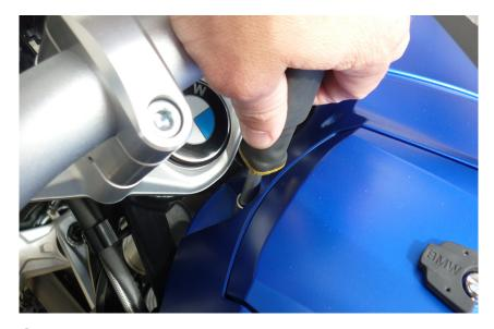
Using T30 driver, loosen the fastener directly behind headstock. You do not need to remove, just loosen.
