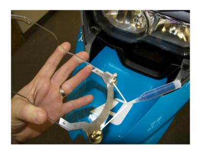
Install ball studs + screws to headlight guard. Hold the guard up to the headlight so you do not mistakenly install the ball studs on the front of the guard. Apply loctite and tighten completely using the 10 mm wrench on the studs flat sides.
