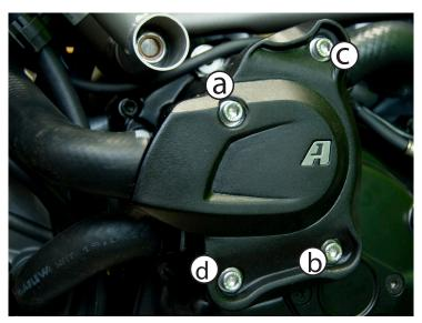
In order to spread the load properly on the gasket, follow the tightening order above. Try to do this in 2 or 3 rounds. Do not tighten each down all the way on the first round. DO NOT OVER TIGHTEN THESE FASTENERS!
