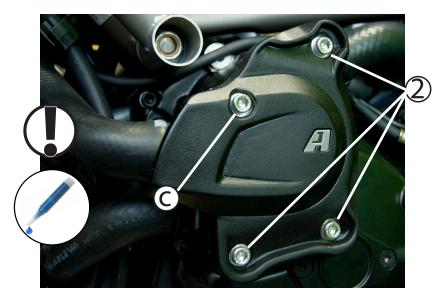
(a)Line up the Guard over the water pump. (b) insert the (4) M6 fasteners w/M6 washers as shown after applying thread locker to the last couple threads of each. (c) is the location of the 50mm long bolt.
